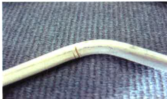
Figure 1. Non-uniform stretching during installation can exert excessive stress on perfluoroelastomer O-rings, even on formed-to-shape seals such as this one.
